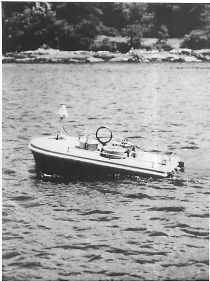
Surface station for a National Ocean Survey (NOS) current meter mooring. Current meter data are recorded on magnetic tape and simultaneously transmitted to a computer aboard the R/V Ferrel.
