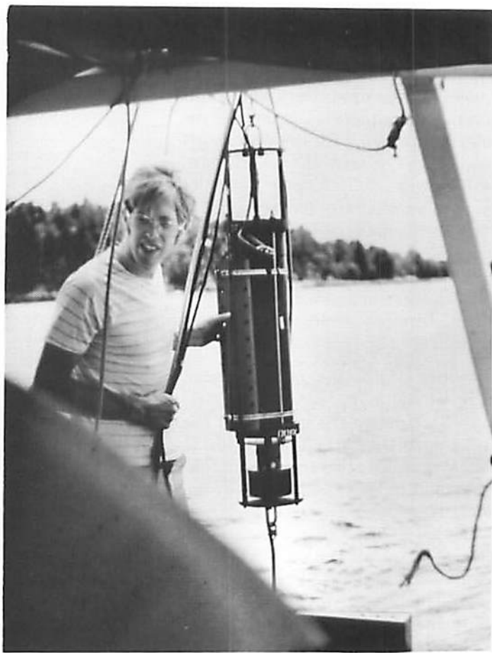
Deployment of a profiling current meter in the Great Bay Estuary. Current speed and direction for each chosen depth are recorded aboard the ship.
