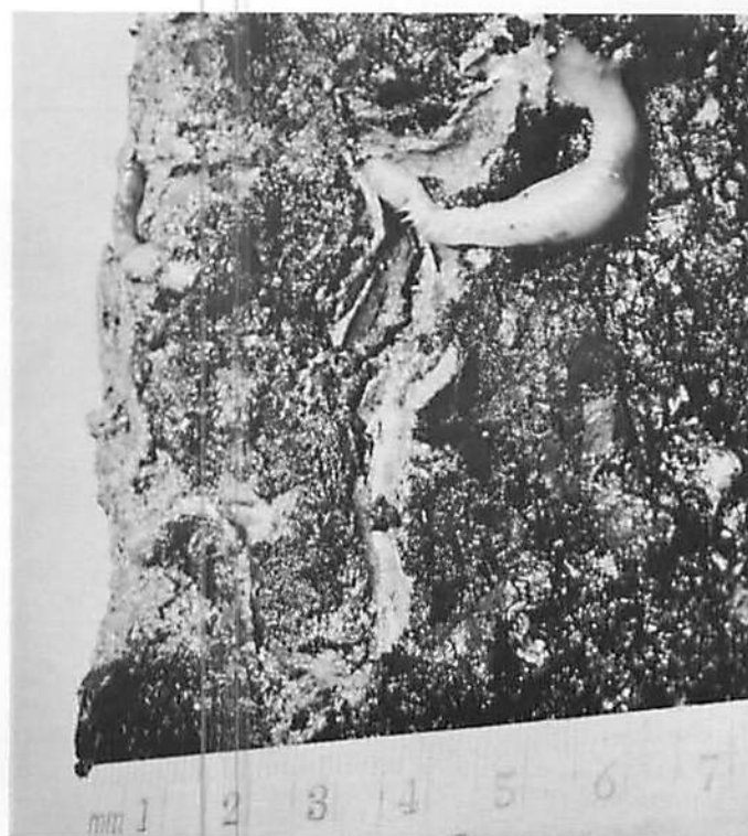
Cross section of a solid waste bale after being submerged for nearly three years. The sabellid polychaete worm shown had penetrated the bale to a depth of nearly 5 cm.
