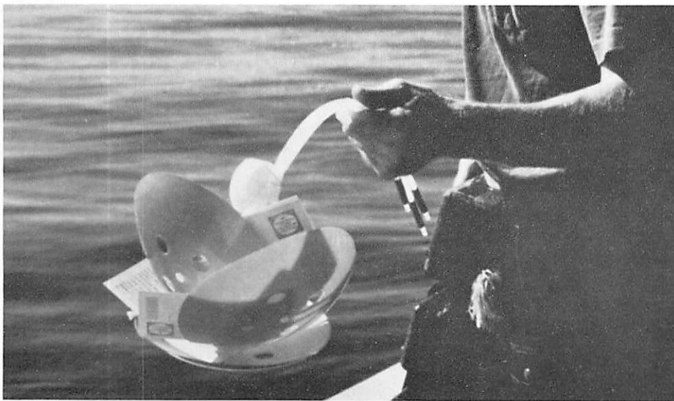
Seabed Drifters Used to Determine the Net Circulation of Water Near the Ocean Bottom. (Note the Spool of Salt to Aid in the Sinking of the Drifter and the Plastic Postal Card Attached to Each Drifter, to be Returned when the Drifter is Found)
