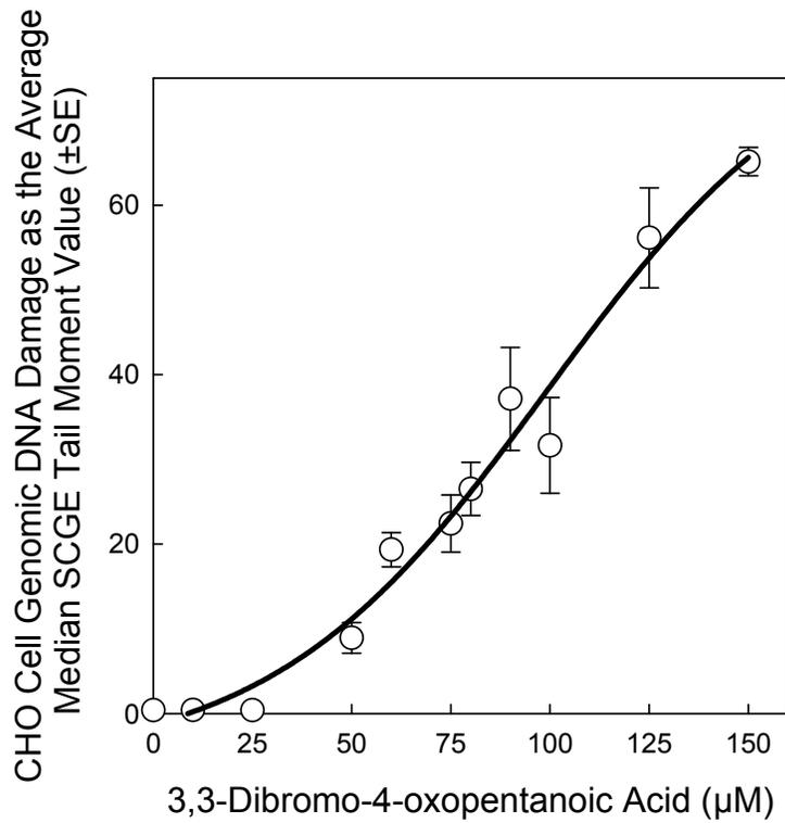
**Figure 5.19 CHO cell SCGE genotoxicity concentration-response curve for 3,3-dibromo-4-oxopentanoic acid**
