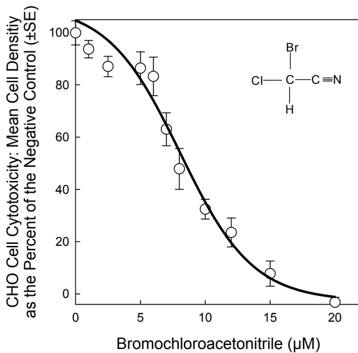
**Figure 6.2 CHO cell chronic cytotoxicity concentration-response curve for bromochloroacetonitrile**
