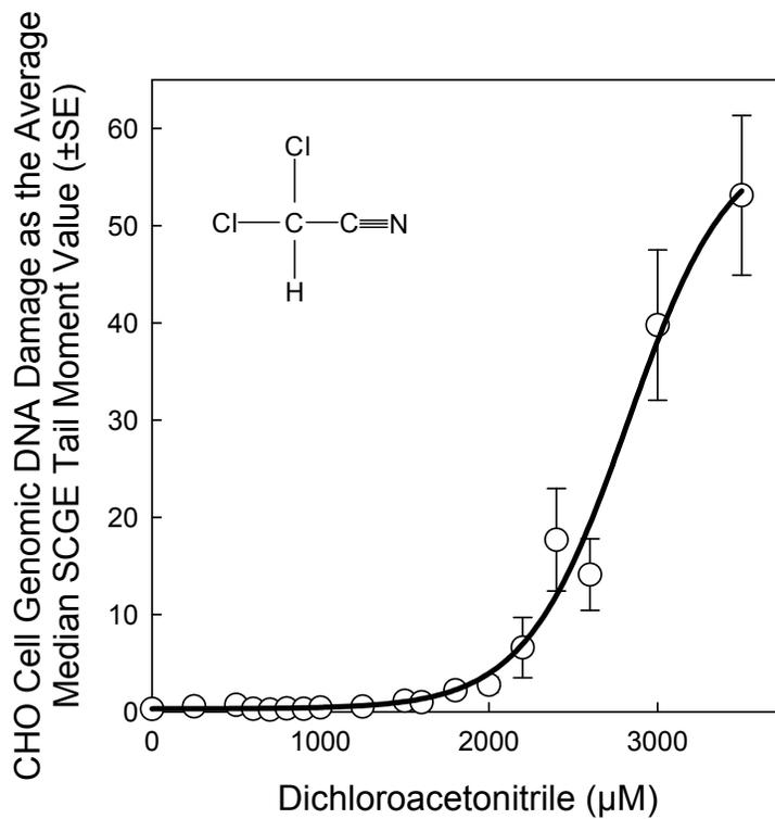
**Figure 6.13 CHO cell SCGE genotoxicity concentration-response curve for dichloroacetonitrile**
