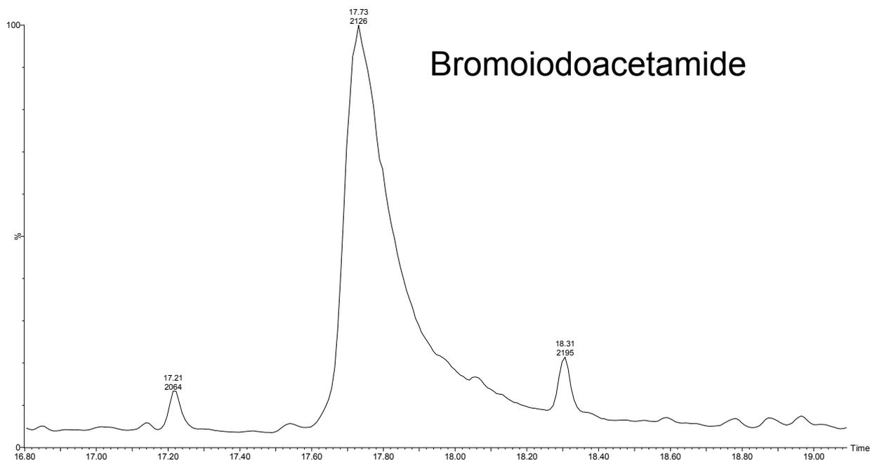
**Figure 7.2 GC/MS chromatogram of a coinjection of bromoiodoacetamide and a drinking water extract**
