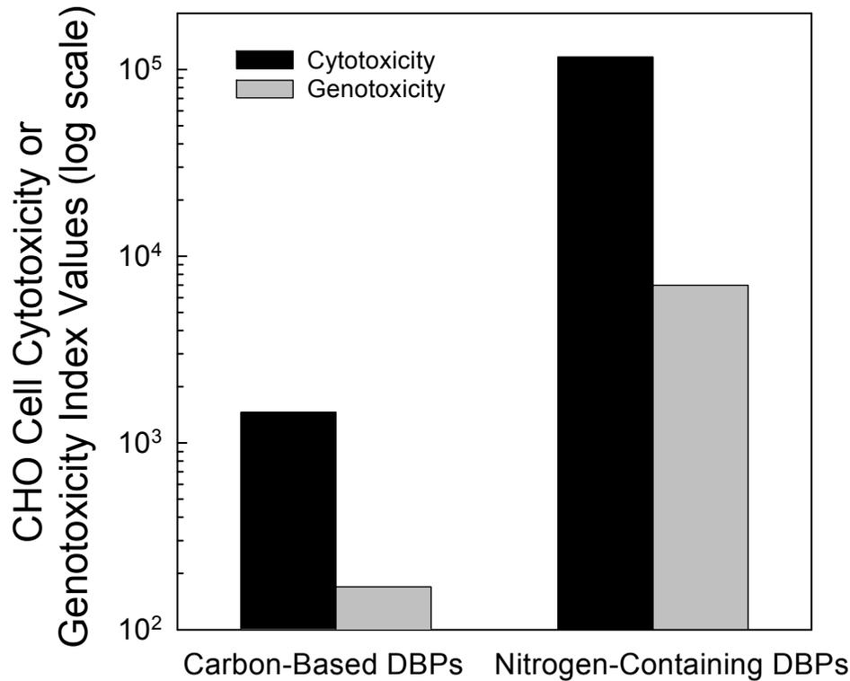
**Figure 9.5 Cytotoxicity and genotoxicity indices for carbon-based DBPs (C-DBPs) versus nitrogen-containing DBPs (N-DBPs)**
