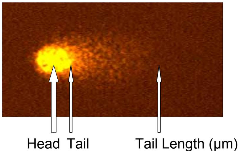
**Figure 2.5 SCGE image illustrating genomic DNA damage in a nucleus. The level of DNA damage is directly related to the amount of DNA that migrates in the microgel (tail). The arrows aid the computer program for the assay that measures the amount and distance of DNA migration.**
