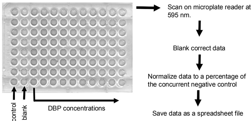
**Figure 2.1** A stained microplate illustrating the CHO cell chronic cytotoxicity assay. The control (column 1) contained cells not exposed to the test compound. The blank column without cells was used to determine the absorbancy of the crystal violet histological dye that was not associated with cells and to normalize the absorbancy data. The DBP or test chemical was assayed from low concentration (column 3) to high concentration (column 12) with 8 replicate cultures per concentration.
