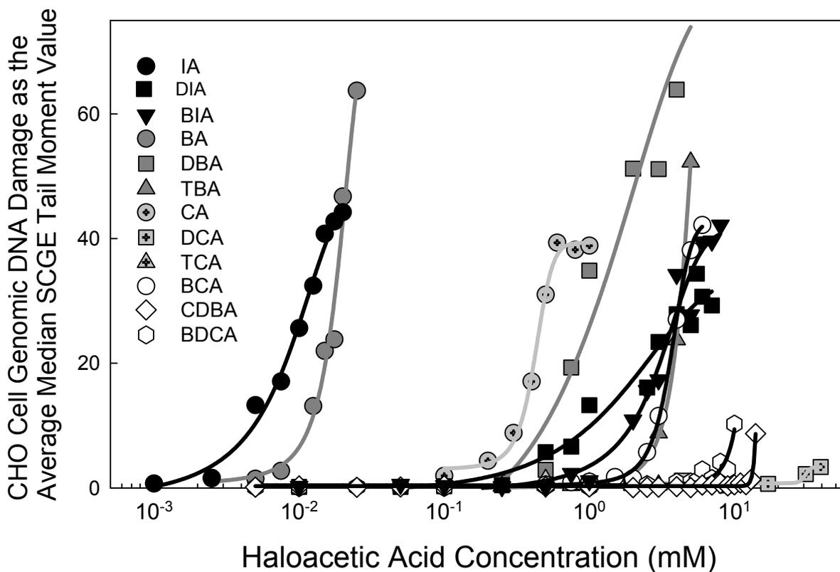
**Figure 4.12 Comparison of the SCGE genotoxicity concentration-response curves of 12 haloacetic acids. The abbreviations are IA = iodoacetic acid, DIA = diiodoacetic acid, BIA = bromoiodoacetic acid, BA = bromoacetic acid, DBA = dibromoacetic acid, TBA = tribromoacetic acid, CA = chloroacetic acid, DCA = dichloroacetic acid, TCA = trichloroacetic acid, BCA = bromochloroacetic acid, CDBA = chlorodibromoacetic acid, and BDCA = bromodichloroacetic acid**
