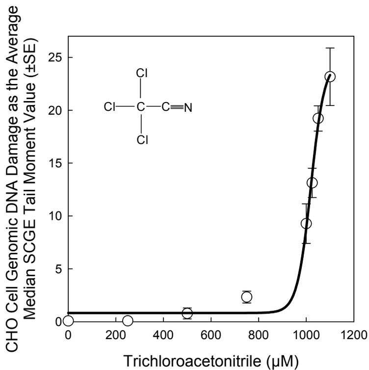
**Figure 6.15 CHO cell SCGE genotoxicity concentration-response curve for trichloroacetonitrile**
