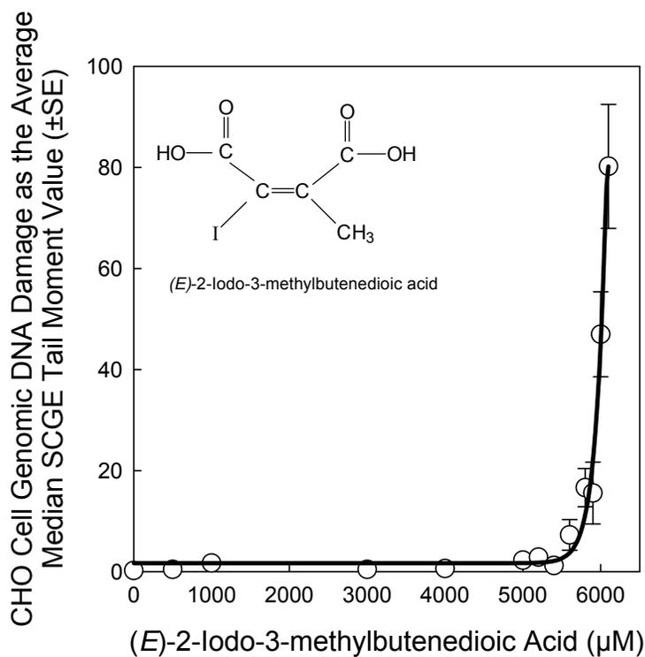
**Figure 5.21** CHO cell SCGE genotoxicity concentration-response curve for (*E*)-2-iodo-3-methylbutenedioic acid
