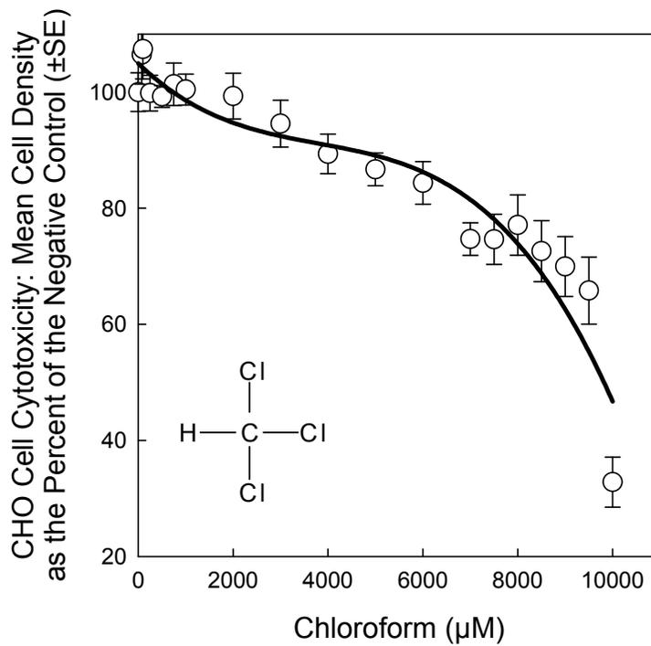
**Figure 3.6 CHO cell chronic cytotoxicity concentration-response curve for trichloromethane (chloroform)**
