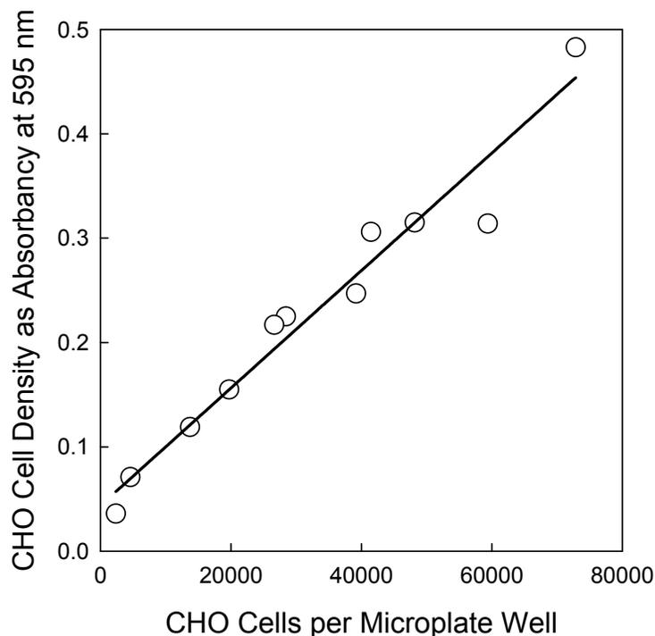
**Figure 2.2** Calibration of the CHO cell cytotoxicity assay. A comparison of the number of cells per microplate well determined by Coulter counting or by the absorbancy after crystal violet staining.
