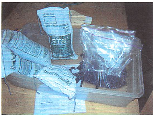
Figure 11: Lead shot application. A. The shot is poured into doubled-up 1 gal. Ziploc bags. B. The bags are placed around the bricks within the cavity.
