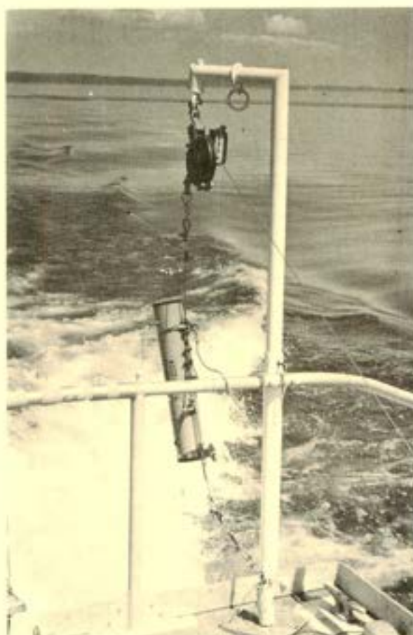
Van Dorn-type water sampling bottle, modified to close 1 meter off the lake bottom. Shown in use aboard R/V Sea Grant I .
