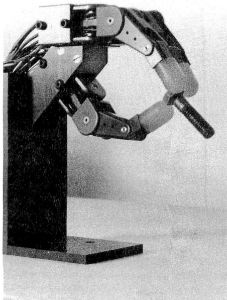
Figure 2. Robot hand can grasp objects, sense the orientation of its fingers, and control its own motion and force.
