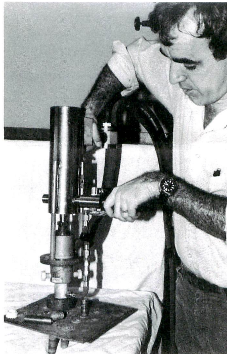
Graduate student Chris Vol Alt demonstrates a prototype of his underwater arc stud welding gun. Diagram shown below.
