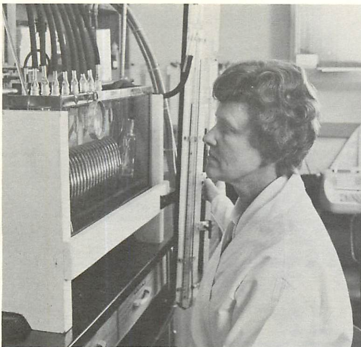
The effects of heavy metal pollution on the respiration of minute larval marine organisms are measured using a Cartesian diver respirometer.
