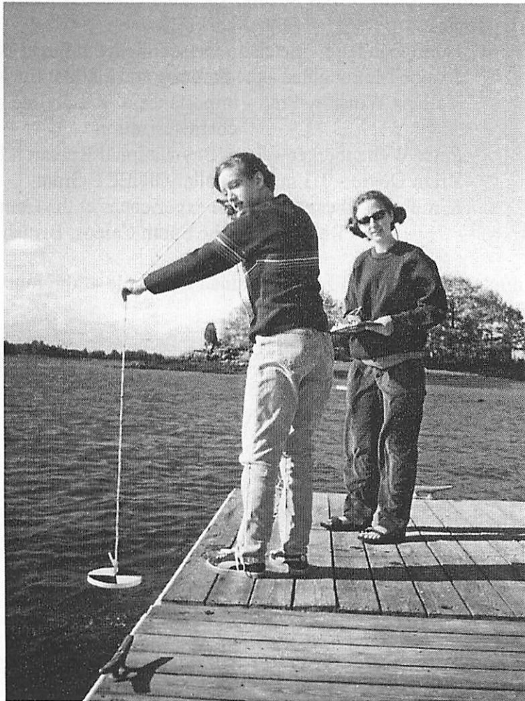
Rachel and Elise Blake measure the transparency and depth with a secchi disk at Site 2, Jackson Estuarine Laboratory.
