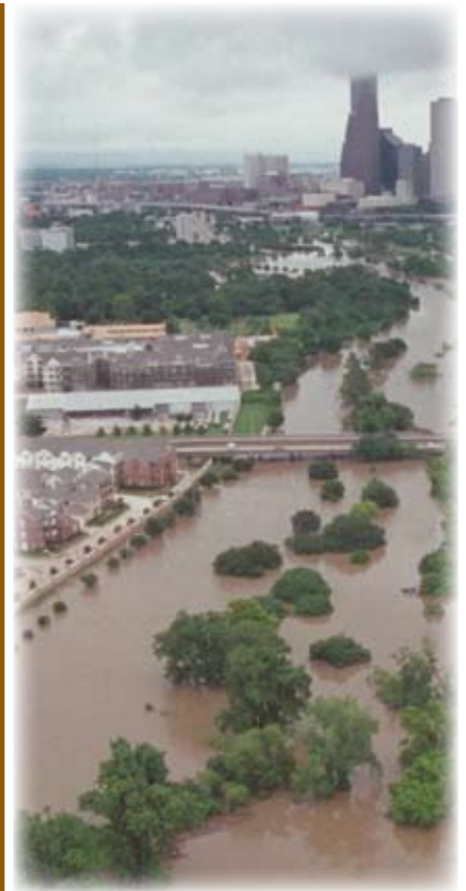
Houston during Tropical Storm Allison. A wide development-free floodplain allows passage of flood waters with little damage in this area.
