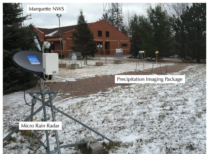
Fig. 2. KMQT instrument deployment configuration.
