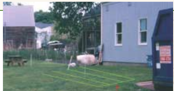
Drawover showing drainfield location
