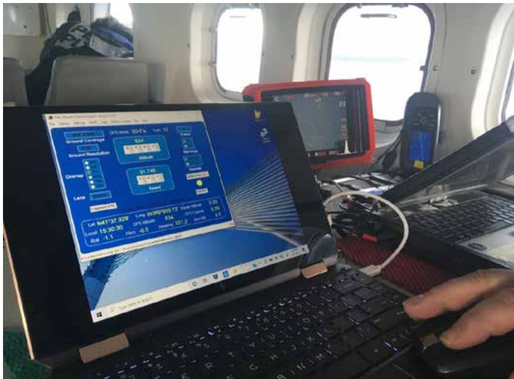
Figure 9-2 Camera system's controller computer (blue screen) and video monitor (red rim)
