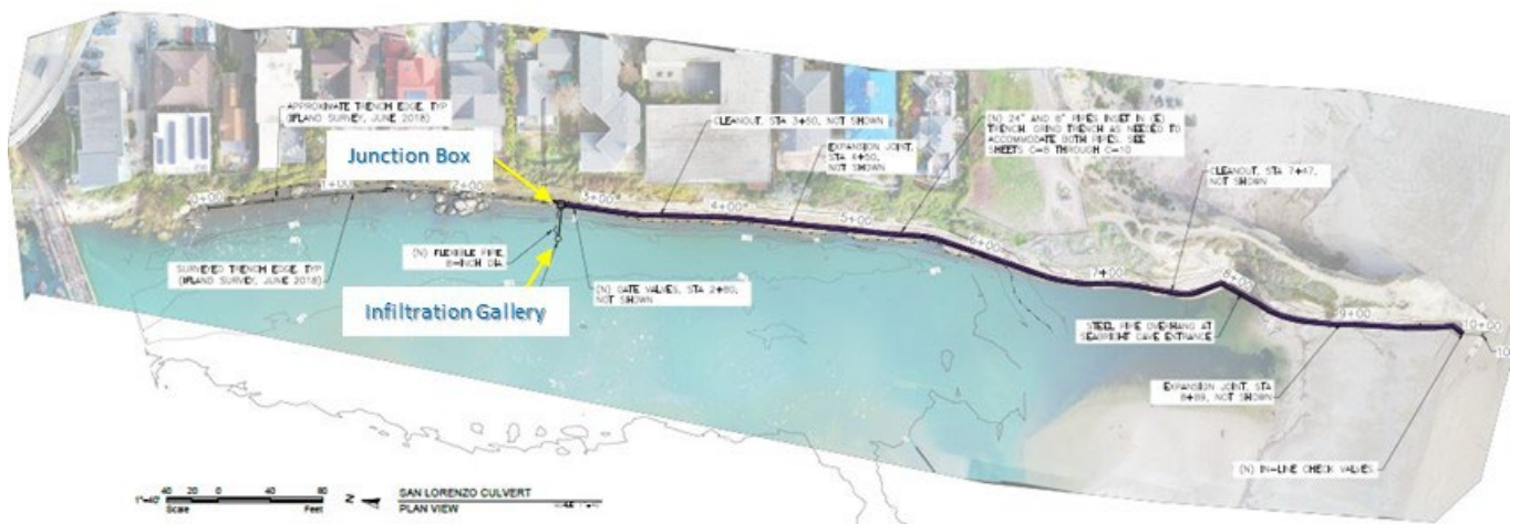
Figure 1. A plan view of the proposed head driven culvert alignment along San Lorenzo Point in the San Lorenzo Lagoon. A portion of the trestle bridge is shown at the far left of the figure with the downstream terminus of the culverts on Main Beach at the right.
