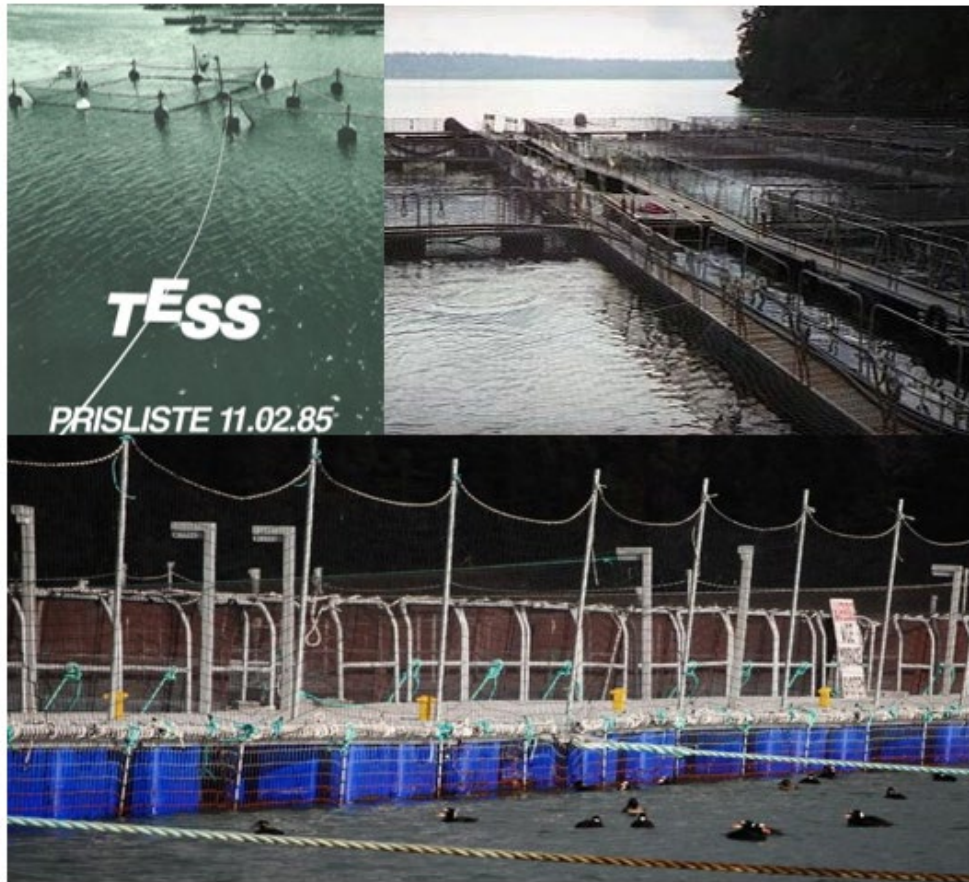
Figure 9. Net pen structures. Top left: 1985 Norwegian aquaculture cage company brochure with early cage technology. Note minimal floatation and no additional predation barrier netting around stock nets. Top right: Example photo of Viking Steel Cage systems which were the second-generation steel pens being developed in the late 1980s to late 90s. Steel cage systems had hinged steel walkways with plastic foam filled floats. Bottom: Outside view of outer walkways showing perimeter predation barrier on the outside of the blue floats lashed tightly to the outer walkway rail used at PS Cooke Aquaculture, Inc. facilities. Predation barrier jump panels are ~7 to 8 ft. above the waterline, and stock net jump walls are ~5 to 6 ft. above the waterline. Bird netting is sewn to the handrails and stretched tightly across the surface of each pen (Parsons 2020).
