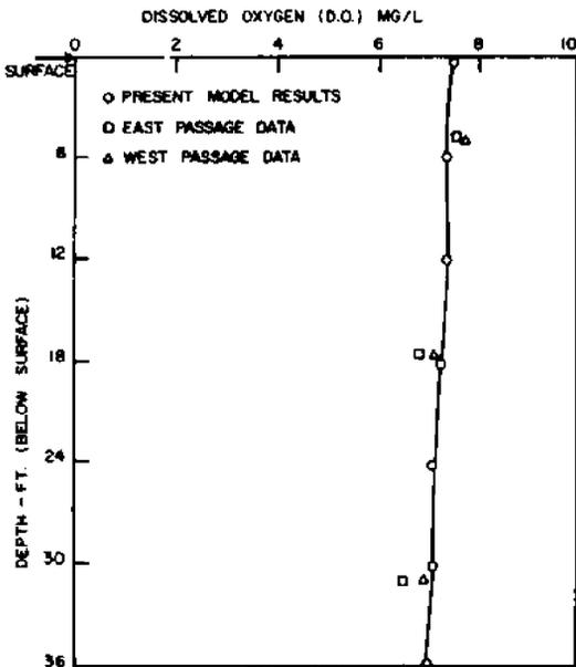
FIGURE 10. Comparison of D.O. vs. depth for data and model results at longitudinal grids 33.
