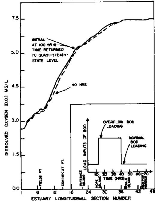
FIGURE 13. Depth averaged D.O. variation caused by overflow B.O.D. loading.
