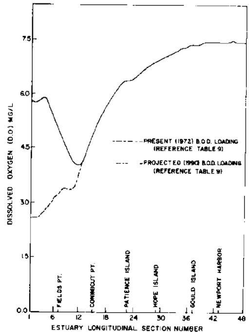
FIGURE 18. Comparison of depth averaged B.O.D. profiles for present (1972) and projected (1990) B.O.D. loading.
