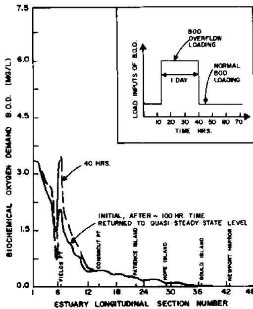
FIGURE 14. Depth averaged B.O.D. variation caused by overflow B.O.D. loading.
