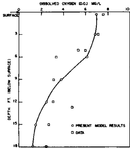
FIGURE 7. Comparison of D.O. vs. depth for data and model results at longitudinal grids 2.
