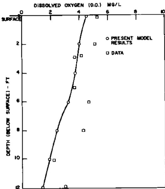
FIGURE 6. Comparison of D.O. vs. depth for data and model results at longitudinal grids 5.
