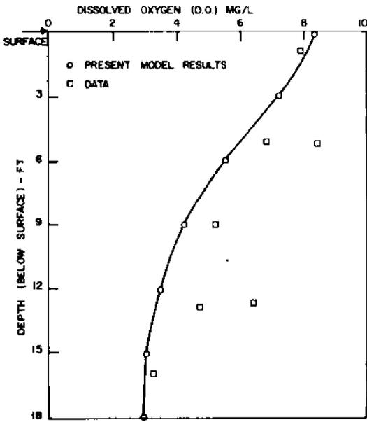
FIGURE 8. Comparison of D.O. vs. depth for data and model results at longitudinal grids 15.
