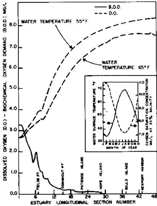
FIGURE 12. Comparison of depth averaged D.O.-B.O.D. profiles for variation in surface water temperature.
