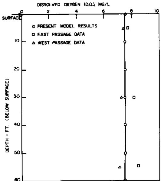
FIGURE 11. Comparison of D.O. vs. depth for data and model results at longitudinal grids 47.
