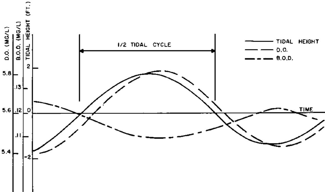
FIGURE 5. Typical variations of D.O., B.O.D. and tidal height for a given location in Narragansett Bay.
