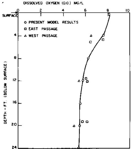
FIGURE 9. Comparison of D.O. vs. depth for data and model results at longitudinal grids 24.
