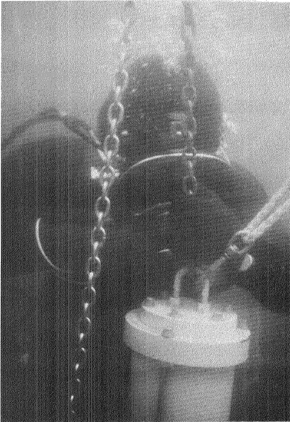
Figure 1-1. Research Diver Equipped with Surface-Supplied Free-Flow/Demand Mask and Variable-Volume Suit Installing a Current Meter for Study of Water Circulation in Grand Traverse Bay (Photo by R. Johnson)
