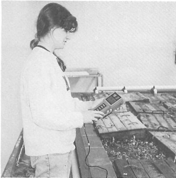
Measuring dissolved oxygen level in water with hand-held oxygen meter
