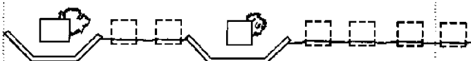
Figure 15. Community approach to shore protection. The community approach reduces the need for flank protection and is more economical and efficient (adapted from US Army Corps of Engineers, 1981a).
