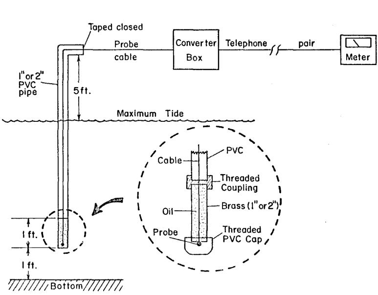
Fig. 3 INSTALLATION DIAGRAM
