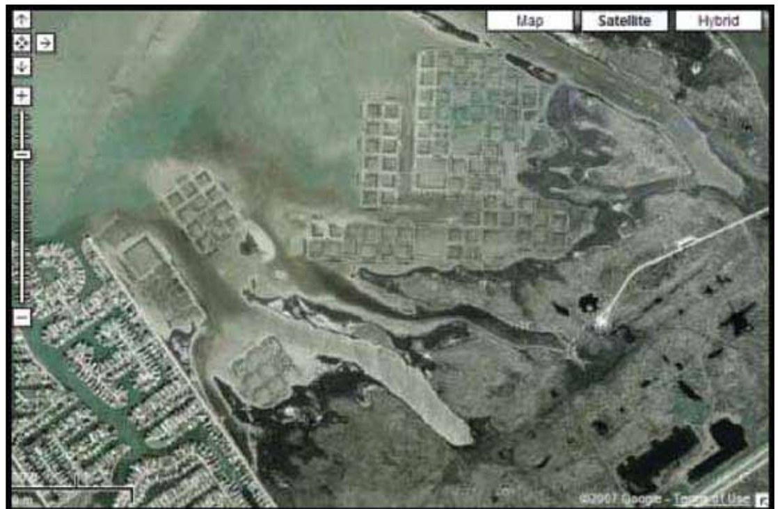
Figure 9. Galveston Island State Park TX. Reticulate grid pattern in upper center of photograph is a complex of wetlands restored to a previously subsided area through the placement of fill material and transplanting of vegetation. The grid provides for maximum edge, the single most important factor in the ecological success of constructed tidal wetlands. Google Maps image captured January 2007.
