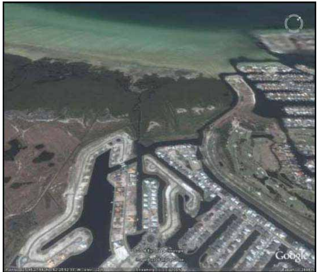
Figure 3. Oblique aerial view of area in Tampa Bay, Florida, showing a classic example of a bulkheaded canal development that impedes landward migration of wetlands. This development appears to have been constructed on high, for-the-most-part non-wetland ground, perhaps impacting few existing regulated wetlands, but in effect destroying inundatable lands just inland of existing coastal wetlands. Bay waters are at top of the photo, with fringing estuarine wetlands just below. Notice that the canal development, in the lower central part of the photo, is relatively recent, with construction still occurring on the left. Image captured from Google Earth, Jan. 5, 2007.
