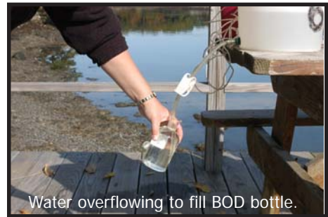
Figure 8.3-2: Properly filling a BOD Bottle
