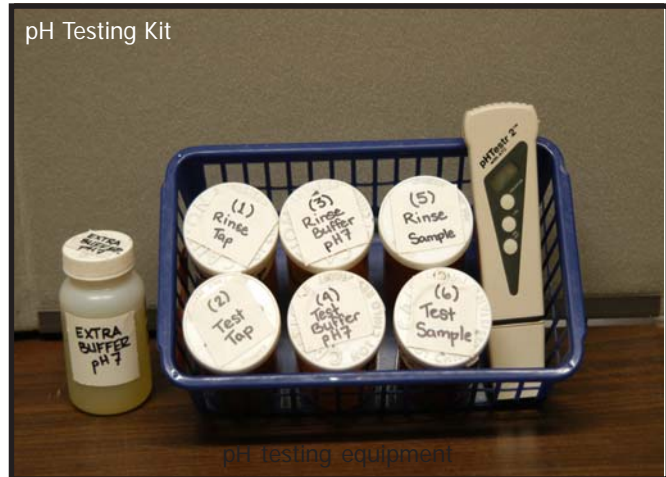
Figure 6.2-1: pH Testing Equipment
