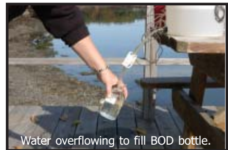
Figure 8.3-2: Properly filling a BOD Bottle
