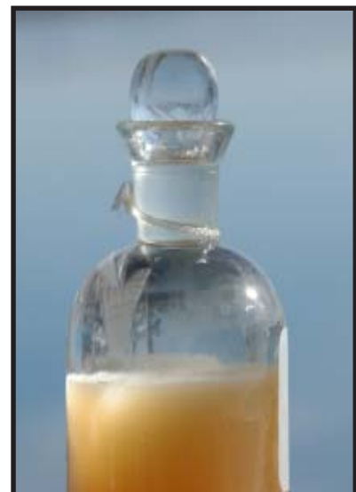
Figure 8.3-3: Settled precipitate in BOD bottle.
