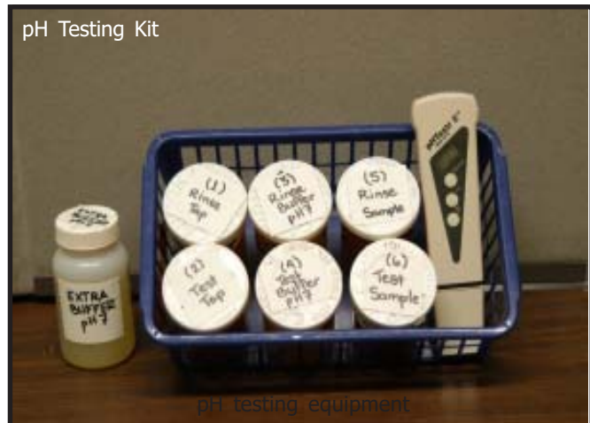
Figure 6.2-1: pH Testing Equipment
