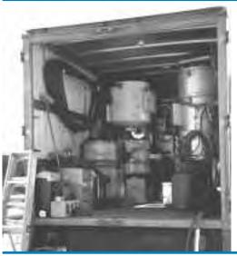
Mobile equipment used to separate and recover plastic blasting media.
