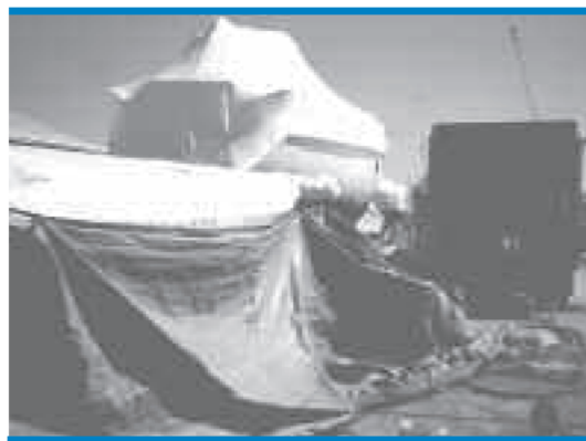
Boat enclosed for plastic media hull blasting.
