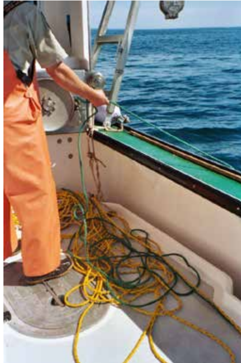
Rope on the deck of the Maine Marine Patrol Vessel Guardian III, showing how rope would accumulate under foot if a rope locker were not available. Photo by Ann Backus, Rockland, Maine 2004.
