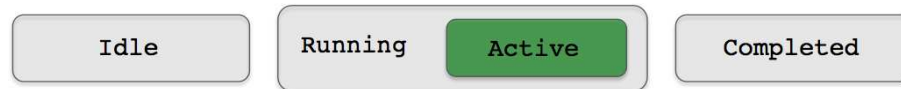
Figure 15: Behavior States: A behavior may be in one of these four states at any given iteration of helm Iterate() loop. The state is determined by examination of MOOS variables stored locally in the helm’s information buffer.
