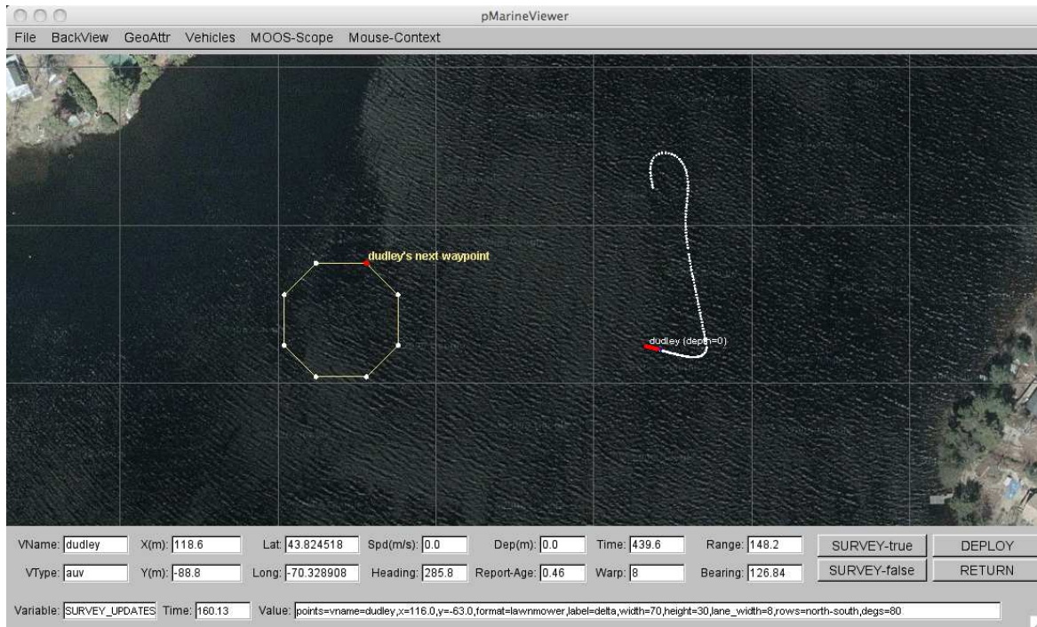
Figure 50: The Delta Mission (3) : Once the vehicle has finished the survey pattern, it re-enters the loiter mode returning to its loiter region. It resumes periodic surfacing and immediately surfaces for a GPS fix.
