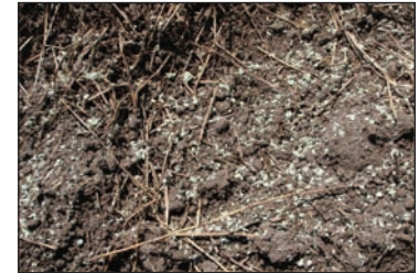
Figure 18: PAM flocculant on soil
