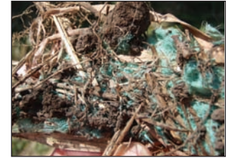
Figure 12: Soil adhering to BFM
