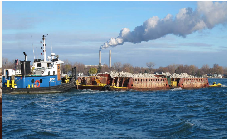
Figure 24. Dump barge used to drop reef material.
