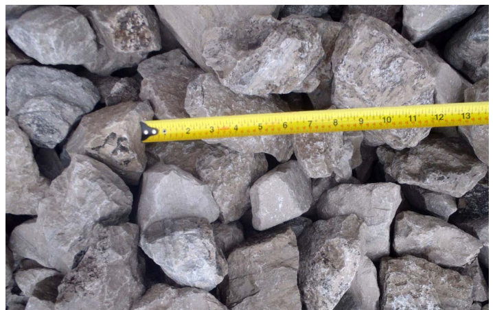
Figure 25. Quarried limestone, 4 – 8 inches in diameter, used for recent spawning reef projects.
