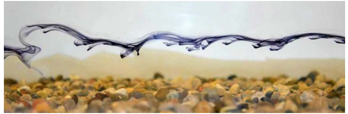
Figure 22. Developing physical and computer models to study water flow over constructed reefs. Credit: Aline Cotel (UM).
