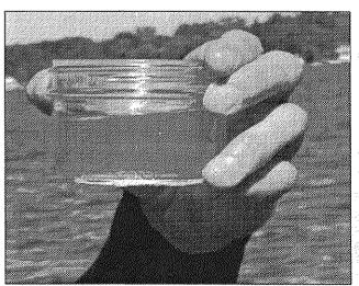
In other words, one sample container should hold the contents of two separate subsamples from one location and be filled to the second mark. Put the lid on the sample container, and set it aside until it is time to add the preservative.
