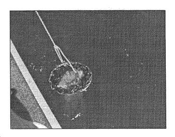
heavy. Let the net sink until the water level reaches the mark on the rope. The bottom of the plankton net—the cod end—will be 18 feet deep.
