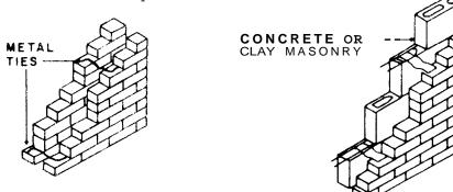
Figure 6 Cavity type walls.
