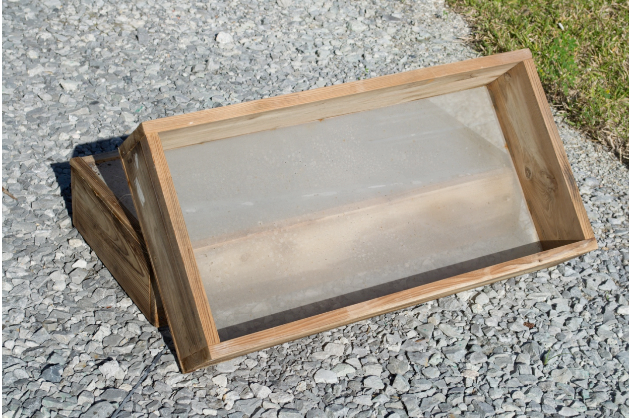
Figure 15. Wooden (cypress) setting tray with mesh bottom (measuring 32" x 16" x 6").
