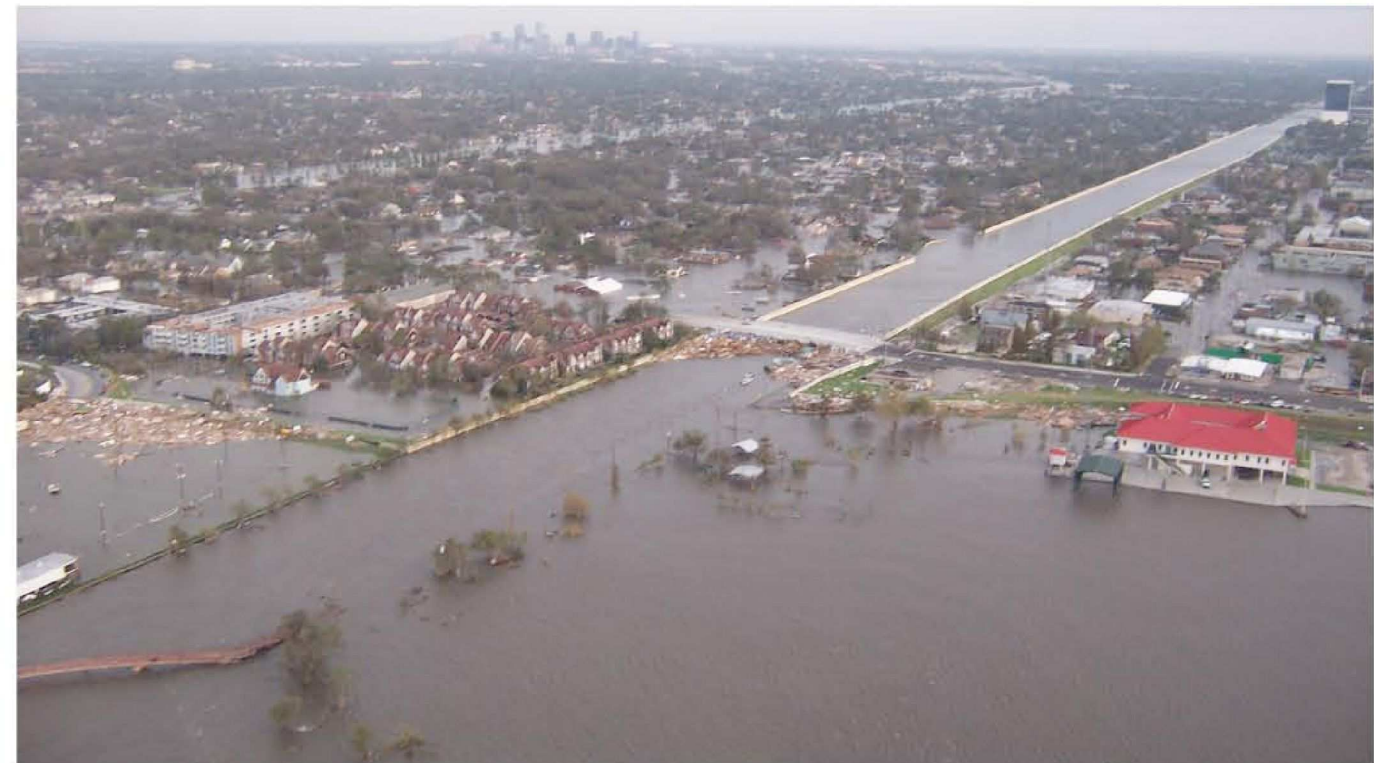
Figure 4-A: Above, a low oblique showing the Coast Guard Station in Bucktown, and the 17th Street Canal levee breach
