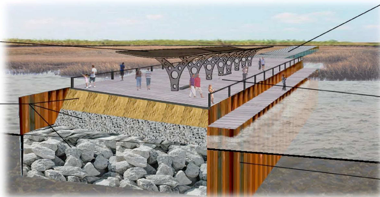
Construction Method for Proposed Pier & Breakwater
