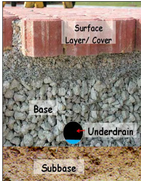
Components of a Permeable Pavement System
