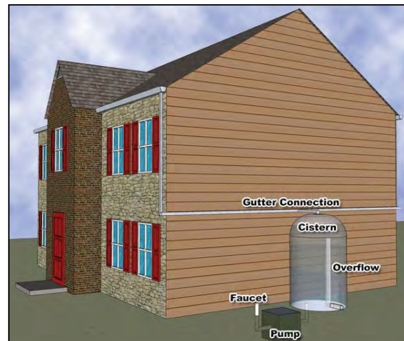
Major Components of a Rainwater Harvesting System
