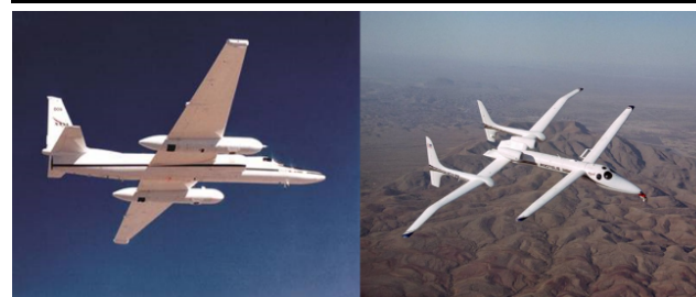
Figure 3. NASA ER-2 (a) and Proteus (b) aircraft used in the MABEL Experiments. Credits: NASA photo
