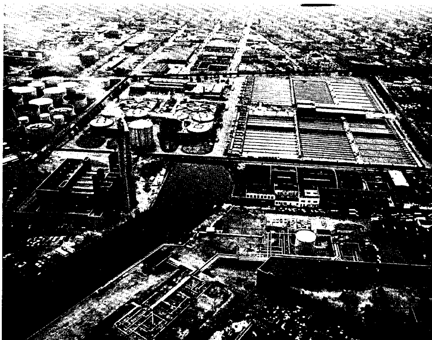
Figure 16. Aerial view of Newtown Creek water pollution control plant, Brooklyn, NY. Foreground channel is tributary to Newtown Creek, which is tributary to East River; thickeners, digesters, sludge holding tanks at left; grit chambers, activated sludge aeration tanks, final clarifiers on right; municipal refuse incinerator in left foreground. (Courtesy of NYC Environmental Protection Administration)
