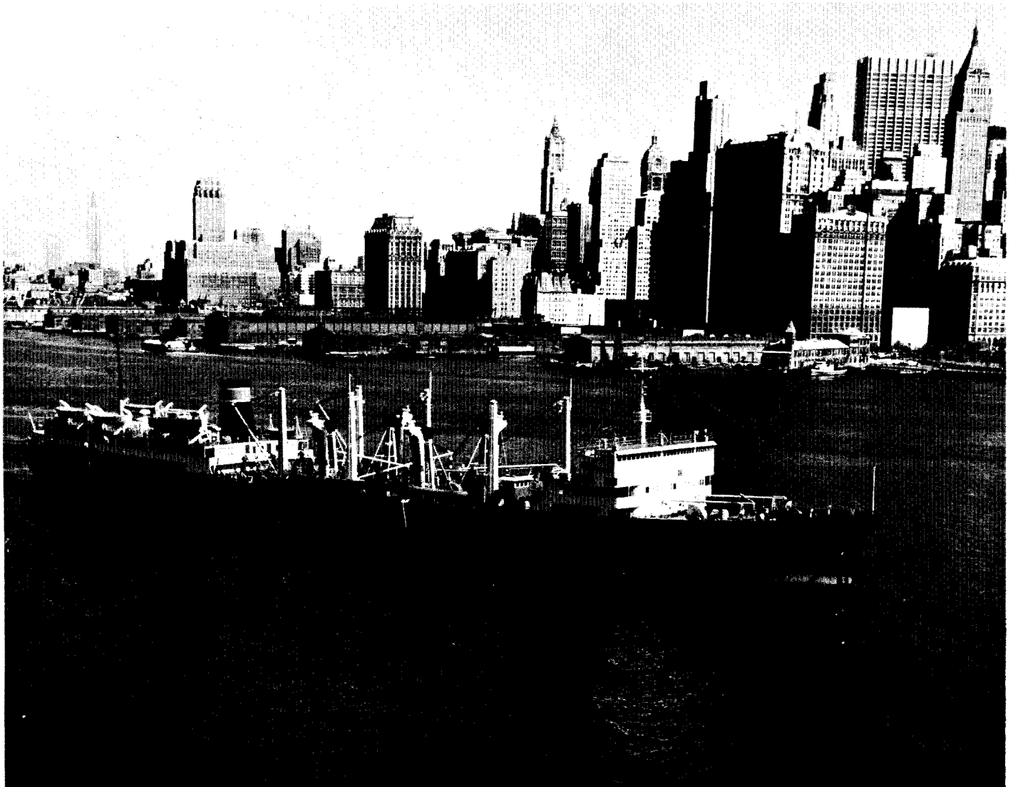
Figure 6. Hopper dredge Essayons : dredges channels in New York Harbor by hydraulic suction and transports material to dumpsite; 525 ft long, 12 hoppers with capacity of 8,270 yd 3 of dredge spoil, displaces 22,410 long tons when loaded (Courtesy of US Army Corps of Engineers, New York District)
