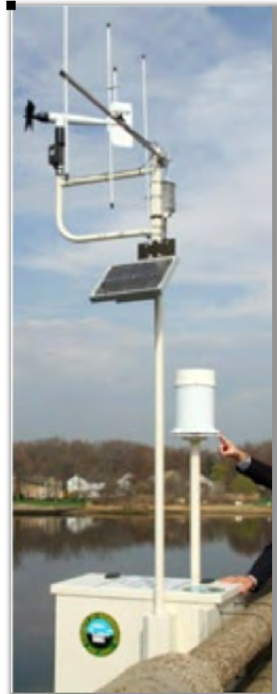
Figure 3.7.1:2 - Shrewsbury River Flood Gauge and Weather Station
