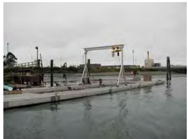
Floating upwelling system used to rear settled larval oysters and clams.
