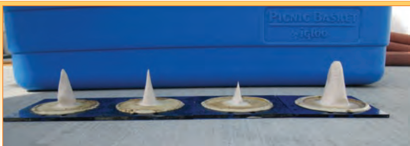
SLODS™ cards measure water flow
