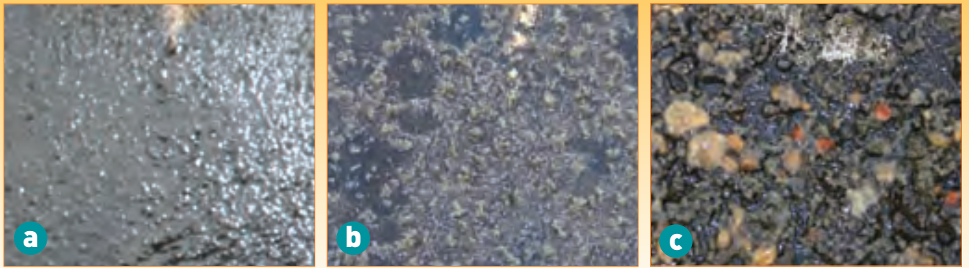
Accumulation of fouling as copper panels age (a) 3, (b) 6 and (c) 12 months
