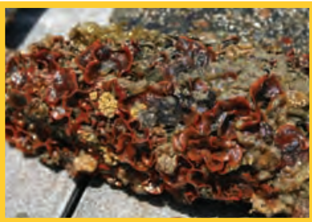
Fouling on experimental panel from San Diego Bay. Note the red "leafy" bryozoan Watersipora subtorquata
