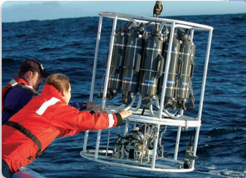
Scientists deploy a rosette of Niskin bottles, used to collect water samples, with a CTD recorder mounted underneath the bottles.
