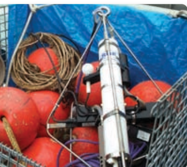
A seawater conductivity-temperature-depth (CTD) recorder. CREDIT: DAVID LEECH, UAF/SFOS
