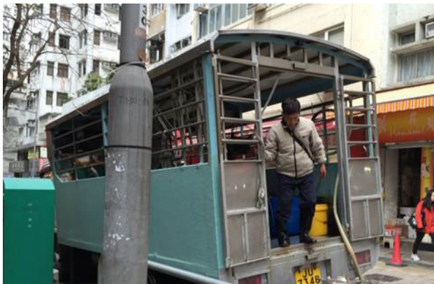
Figure 4.32. Live fish delivery trucks. Live seafood is delivered to retail and/or restaurant establishments by open-top trucks equipped with air hoses to aerate the fish. Fish are put in plastic tubs filled with freshwater or seawater, depending on species.
