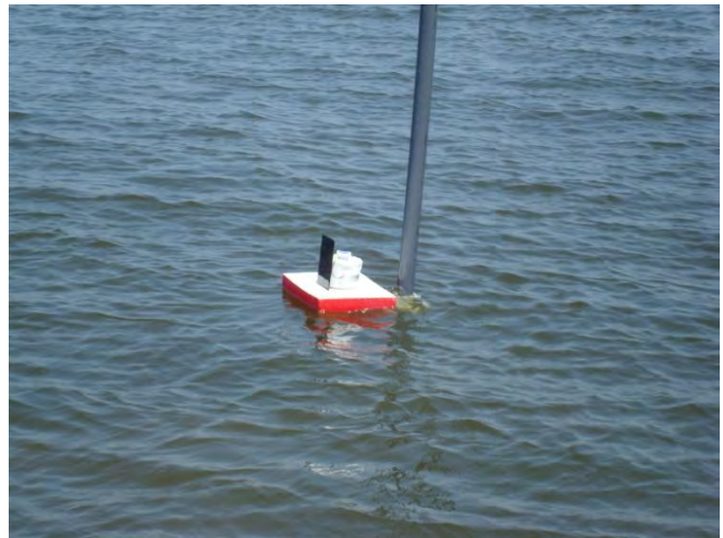
Figure 3. Close-up of DRIFTER module deployed near Half Moon Island.
