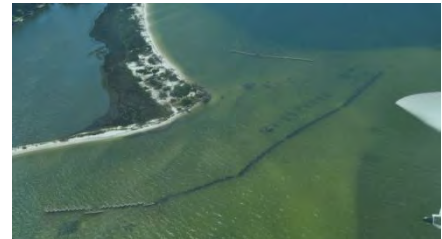
Figure 1- A 2011 aerial photos showing the two types of breakwaters protecting Deadman's Island, Gulf Breeze, Fla.
