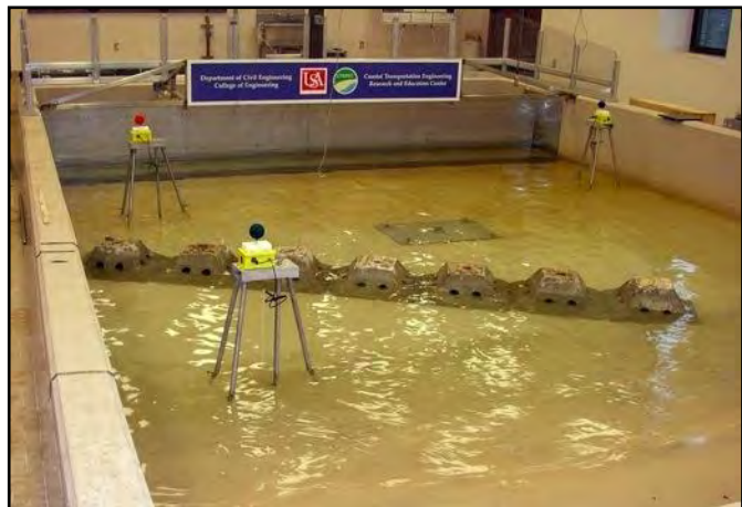
Figure 1. Laboratory testing of wave transmission through concrete wave attenuation devices in the USA Coastal Transportation Engineering Research and Education Center wave basin.
