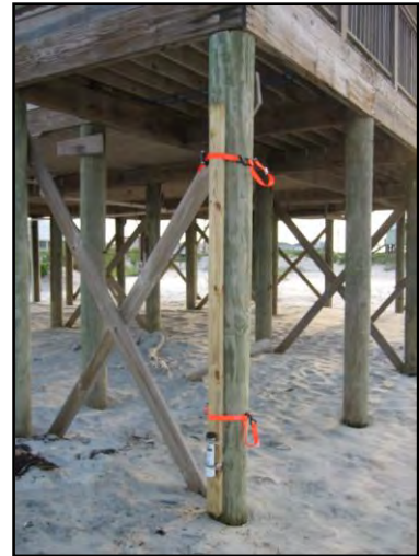
Figure 1. A storm surge and wave gauge deployed on Dauphin Island, Ala.
