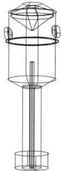
Figure 1. The buoy is made of aluminum, and shows the shell with the feed pipe and hopper.
