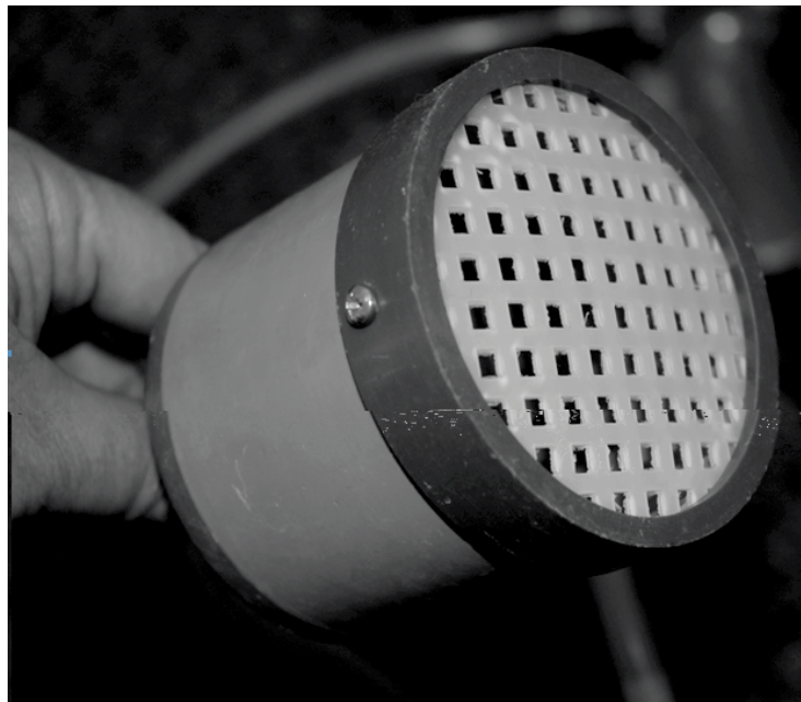
Figure 6. Air diffuser for the pneumatic wrench. Photo credit: Stephanie Schwabe.
