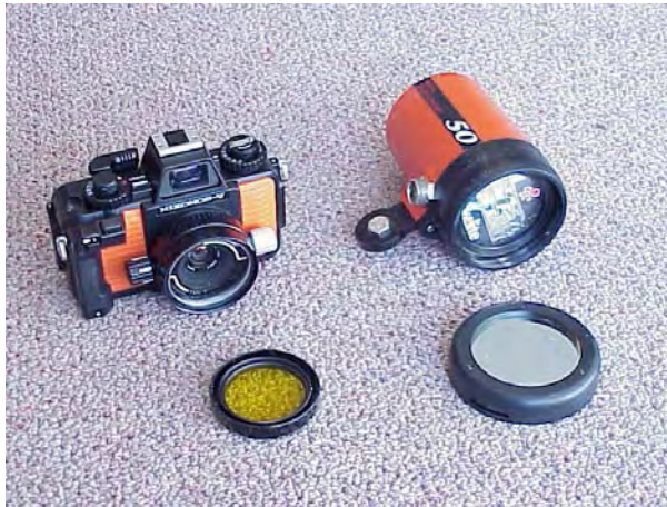
Figure 4. Nikonos V underwater camera and Ikelite underwater flash, showing the barrier and excitation filters that would be used with each.
