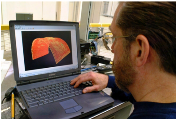
Examining a laser scan of an exterior hull plate. Copyright Friends of the Hunley.
