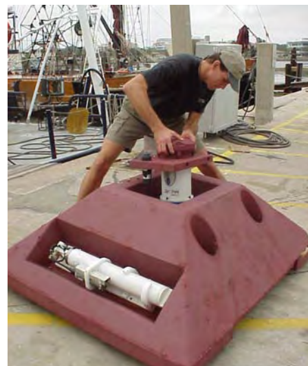
Figure 2: Rick Cole prepares a bottom mount with ADCP and SeaGauge for deployment)
