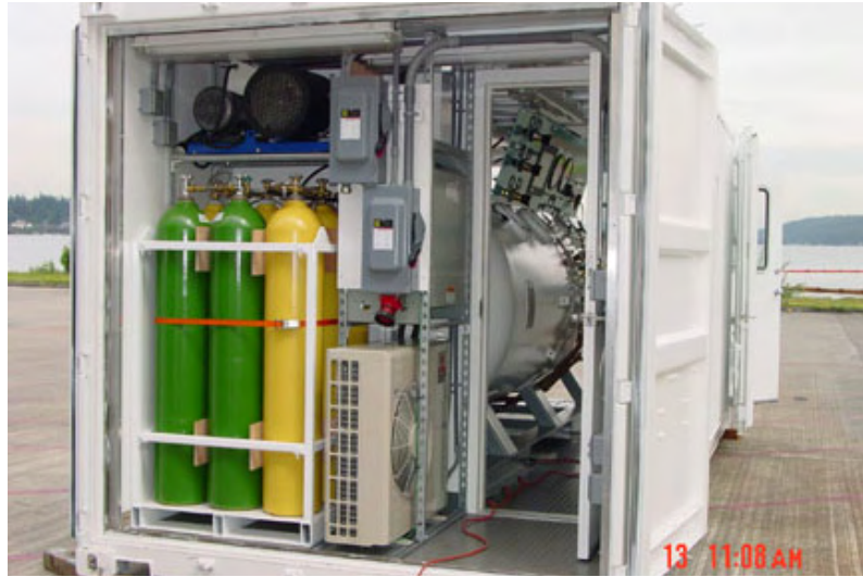
Figure 10: Containerized recompression chamber
