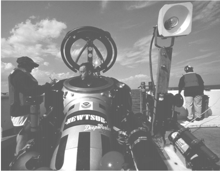
Figure 1. A Deepworker 2000 one-person submersible. Note the video and still camera at lower right. The sector-scanning sonar head is to the left of the hatch. A Li-Cor quantum light sensor to measure downwelling light was mounted astern of the hatch. The submersible used two 250 watt quartz and two 100 watt HID lights for illumination.
