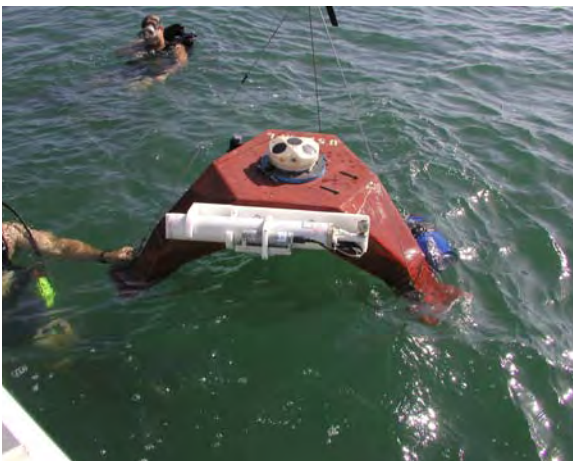
Figure 11 Acoustic Wave Gauge deployment
