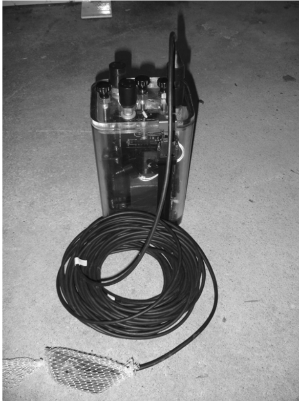
Figure 5 Photograph of the author's first "spawn-o-meter" device for recording fish sounds without scuba diver bubble interference. This first generation spawn-o-meter was built and deployed in 1989 and included a hydrophone (foreground) connected to a tape recorder in an underwater housing with controls. It was equipped with up to two hydrophones for stereo recording and an earphone for real-time listening option. Such autonomous recorders are deployed at a site where fish are active and then the diver leaves the area to avoid bubble interference. These can be programmed to record at various time intervals. Hydrophones are omni-directional and thus all fish sounds within several meters or more (depending on the source level) are recorded. Deployment of such devices underwater qualifies as "tactical diving". The key to obtaining meaningful data is to know where, when and how to deploy your data acquisition diver/apparatus.
