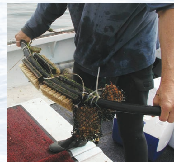
Common scrub brushes have proved to be efficient and cost-effective collectors to study larval settlement in marine field studies. photo: courtesy of Dr. Steve Schroeter
