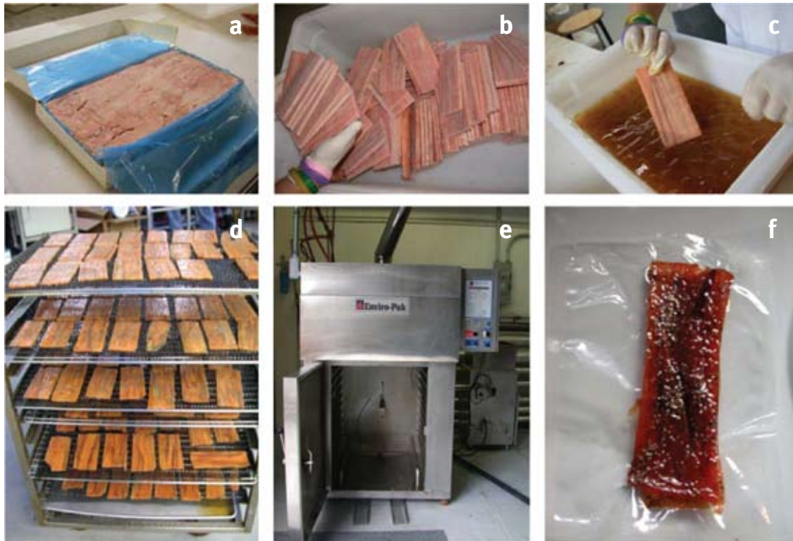
Figure 1. Representative steps for the manufacturing of salmon jerky from salmon blocks: (a) Pink salmon block; (b) Frozen salmon strips; (c) Glazing salmon strips; (d) Glazed salmon strips on the smoking cart (5 trays depicted); (e) Smokehouse; (f) Individually vacuum packaged salmon jerky.
