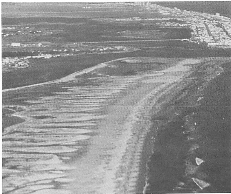
Fig. 2.8. A striking example of island migration. The jetties built at the south end of Ocean City, Maryland (top of photo), caused sand starvation of adjacent Assateague Island. In the early 1930s the 2 islands formed a more or less straight line.
