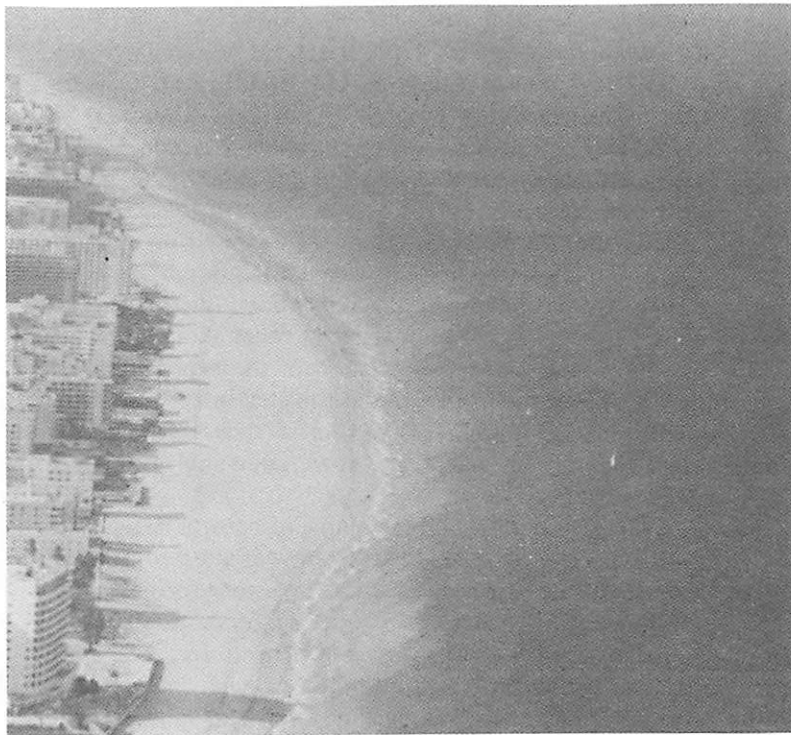
Fig. D-10. Oblique aerial view north along Miami Beach in May 1980, just after the major beach fill. Note the murky water just seaward of the new beach.
