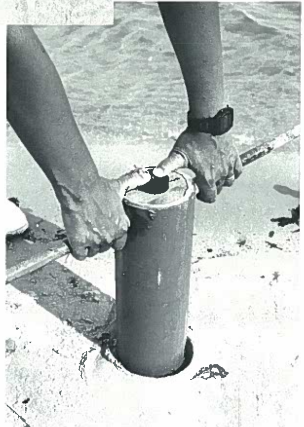
Figure 2. Demonstration of core tube on sand beach for demonstration only. (Top) 4-inch diameter PVC core tube with 1-inch PVC tube installed and sealed. Removable metal handle inserted in tube for coring. Rubber stopper loose on top for insertion into sediment. Note beveled lower edge of 4-inch tube to aid in cutting rhizomes. (Right) Core tube after twisting into sediment to depth of ca. 20 cm. Rubber stopper is in place in plywood plug that was screwed in place and bedded in sealant. Placement of the stopper creates a vacuum that allows the plug of seagrass to be withdrawn from the substrate. Removal of the stopper allows the plug to slide out of the tube into the substrate for planting.
