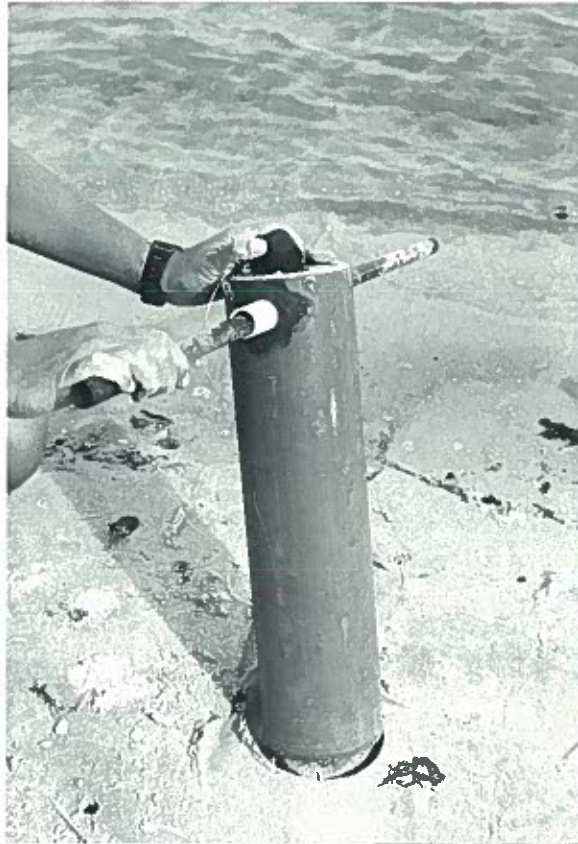
Figure 2. Demonstration of core tube on sand beach for demonstration only. (Top) 4-inch diameter PVC core tube with 1-inch PVC tube installed and sealed. Removable metal handle inserted in tube for coring. Rubber stopper loose on top for insertion into sediment. Note beveled lower edge of 4-inch tube to aid in cutting rhizomes. (Right) Core tube after twisting into sediment to depth of ca. 20 cm. Rubber stopper is in place in plywood plug that was screwed in place and bedded in sealant. Placement of the stopper creates a vacuum that allows the plug of seagrass to be withdrawn from the substrate. Removal of the stopper allows the plug to slide out of the tube into the substrate for planting.
